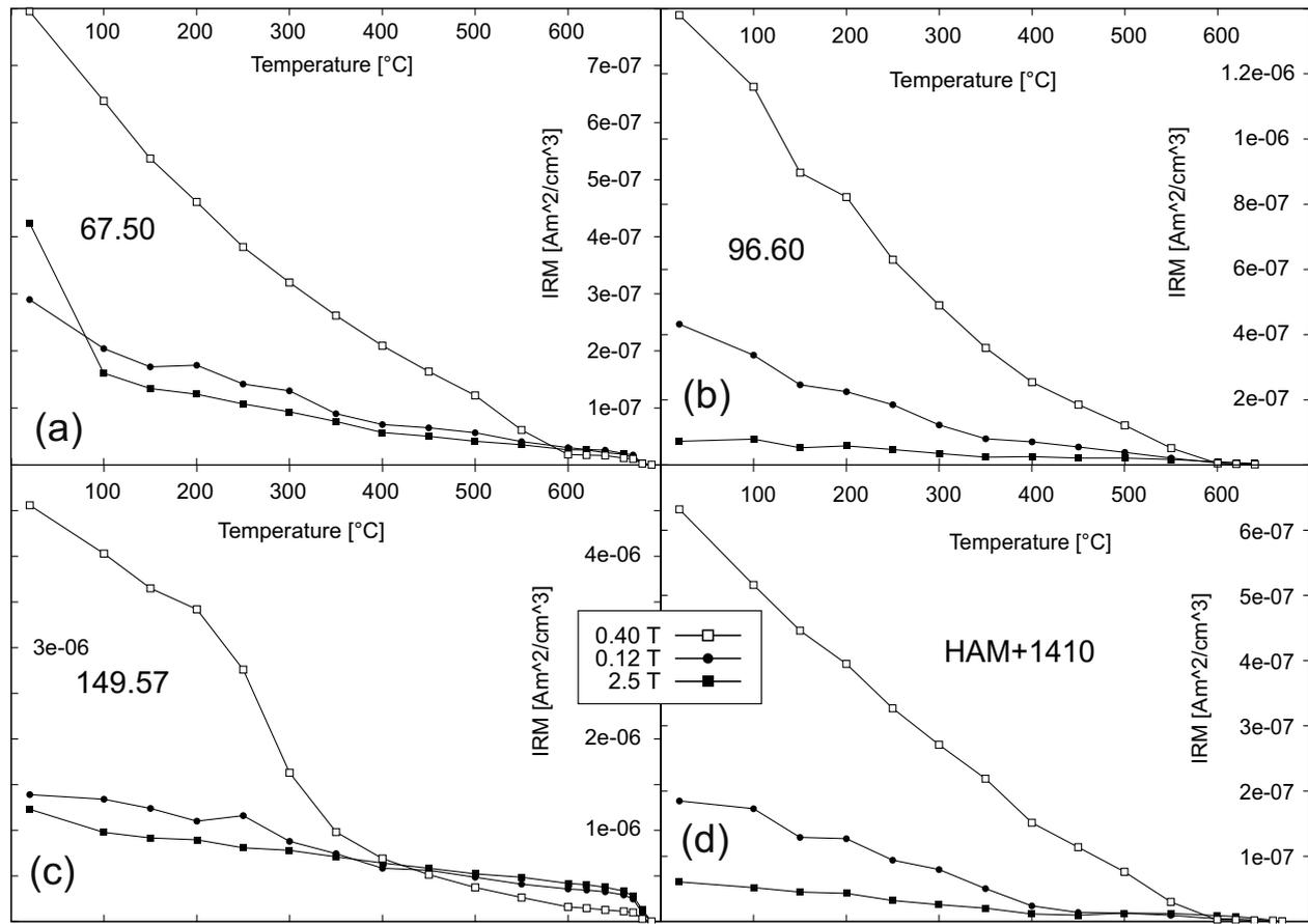
**Fig. 4.** Results of stepwise thermal demagnetization of a composite three axis isothermal remanent magnetization (IRM) with fields of 0.12, 0.40 and 2.5 T (Lowrie 1990) of four representative samples of each section. (a–c) show samples from the Irsee drill core, where the sample name corresponds to the stratigraphic position below surface. (d) shows the result of a sample from the Hammerschmiede section.
